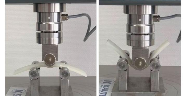
*Example of bending test phases on a pinch-off sample of a PA11 liner after blow moulding production*
