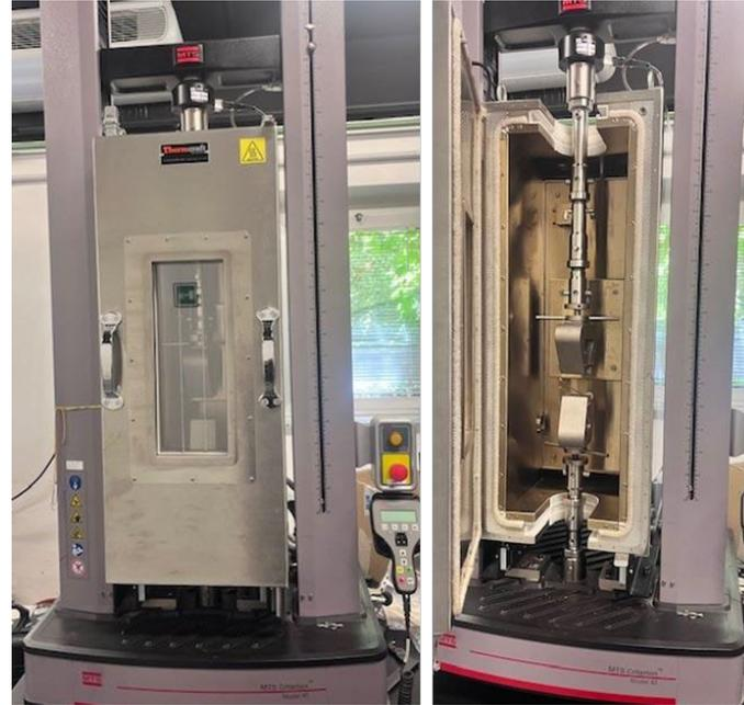
*Tensile testing apparatus with climatic chamber*
