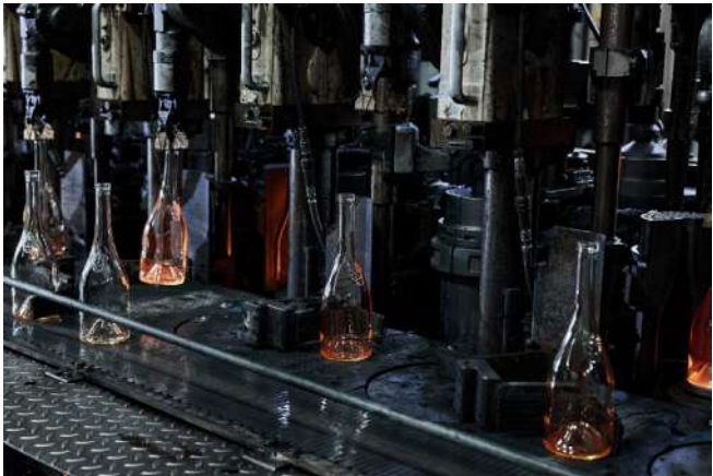
Production of premium glass bottles during trial operation of the oxyfuel furnace utilizing hydrogen as the fuel source.
