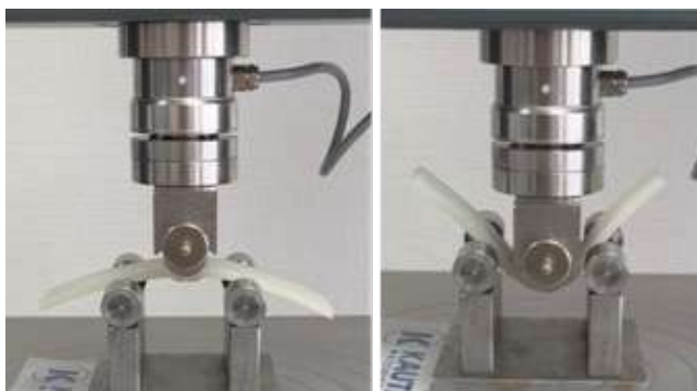
Example of bending test phases on a pinch-off sample of a PA11 liner after blow moulding production
