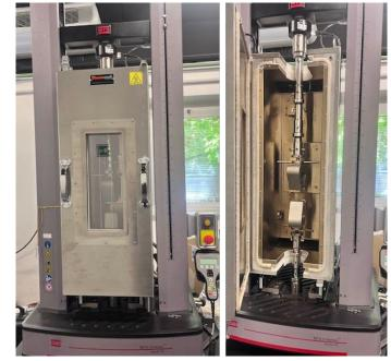
Tensile testing apparatus with climatic chamber
