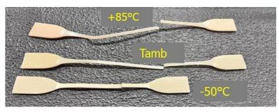
Example of PA6 samples after tensile test at different temperature conditions
