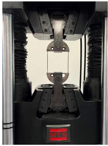
Composite ring during tensile test
